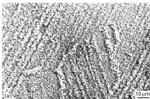
Figure 4 Scanning electron micrograph of a cross-section of a Ti-46.6%Al, 1.9%Cr, 1.8%Nb, (0.127-0.3)%Fe alloy oxidized for 100 h at 800 °C; (a) secondary image, (b) backscattered image.
